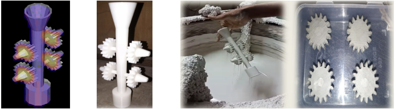
Fig. 7 Thermal simulation and processing of gears using investment casting and 3D printing technology
