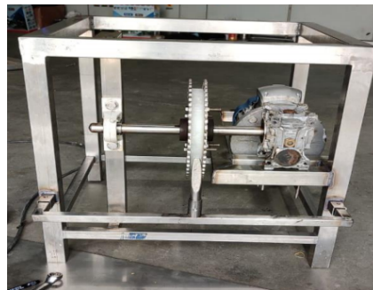
Fig. 6 Design and development of deshelling machine to obtain coconut fruit. (The project was done by the student's group Gandhi Shilp (17PE416), Kashyap Thacker (17PE418) Pritul Makadia (17PE421))
