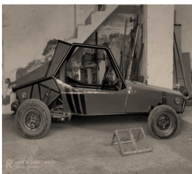
Fig. 3 Pre-assembled ATV made from scrap and its tie rod adjustment for correction in turning radius
